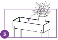
**Step 3** Position your garden planter and fill with plants. *Tip: Built-in adjustable feet* can be raised or lowered on uneven surfaces; use planter pots so you can quickly & easily swap out plants.
