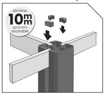
Cut your slats to fit snuggly between the posts and insert them with spacers as required. Use a spirit level to ensure that your first (bottom) slat is level.
