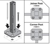
Mark & drill the four anchor holes, noting fastener positions shown above. Secure the base plate to the ground surface with suitable bolts or screws.
