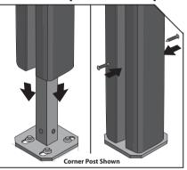
Use spirit level to ensure the base is plumb and level. Slide the post over the base plate and secure in place with screws provided. Double check the levels.
