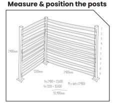
Plan and mark the position of your screen. Measure the distance between posts and check heights so you can determine materials needed.
