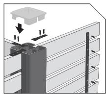
Lock in top slat with bracket and 2 screws. Mark and drill holes in the brace strip to line up with the back of each slat. Fix in place with 15mm button-head screws. Replace cap.
